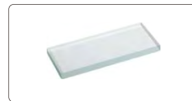
50mm reading scale (check magnification accuracy)
