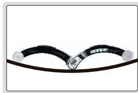
internal diameter measurement
