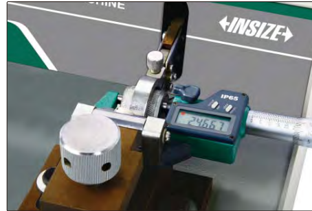
lapping measuring surfaces of outside micrometer
