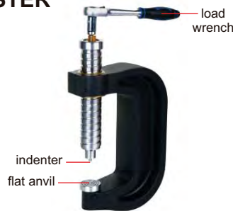
static test clamp
