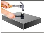
hammer impact to apply test force
