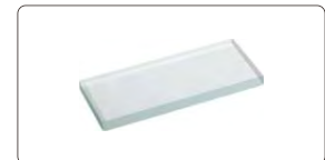
50mm reading scale (check magnification accuracy)
